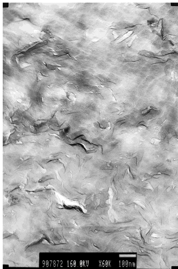
Figure 2. TEM micrograph of the PAN filled with 5 wt % o -PK805.
